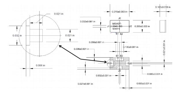
Note: Metalized area on backside is the RF, DC and Thermal ground. In user's end application this surface temperature must be managed to meet the power handling requirements.
